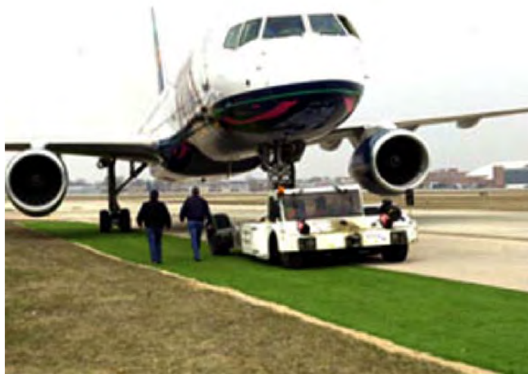
FIGURE 4-3. FULLY FUELED B-757 TAXIING ACROSS ARTIFICIAL TURF SURFACE (BOS)
