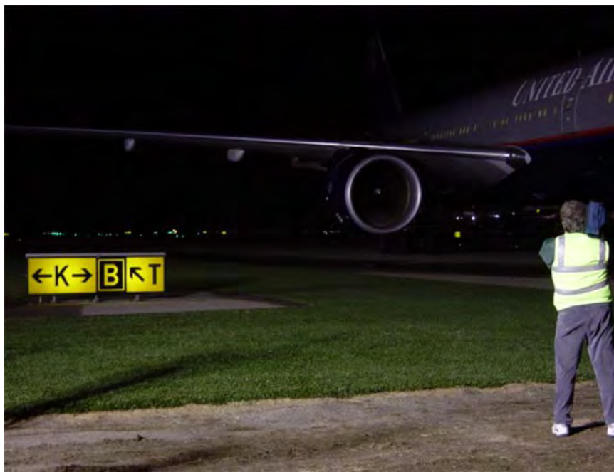
FIGURE 4-9. BOEING 777 TAXIING BY ARTIFICIAL TURF (JET BLAST TEST ACROSS ARTIFICIAL TURF SURFACE) (SFO)
