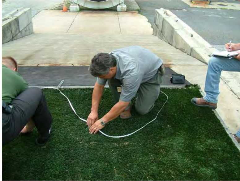
FIGURE C-2. MEASURING SAND MOVEMENT AFTER TEST RUN
