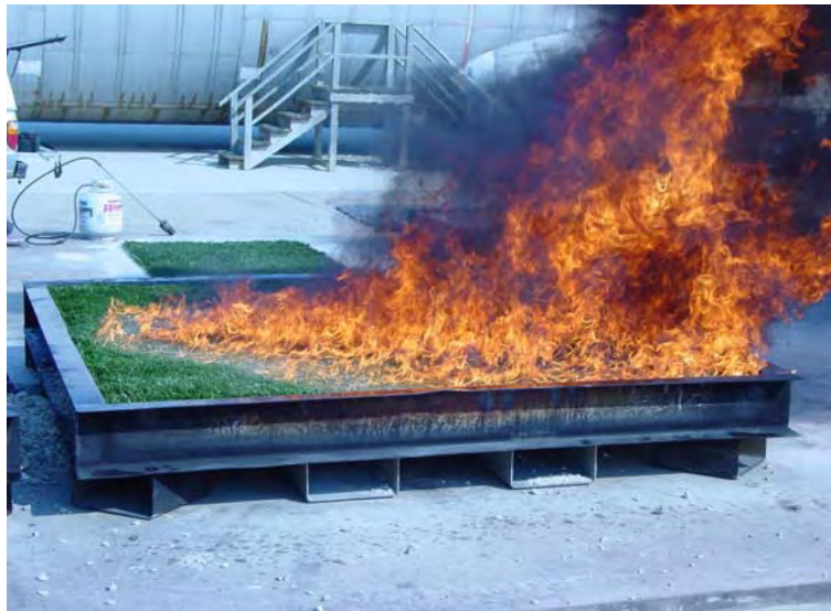
FIGURE D-19. LARGE PAN FIRE—20 GALLONS OF JP-8
