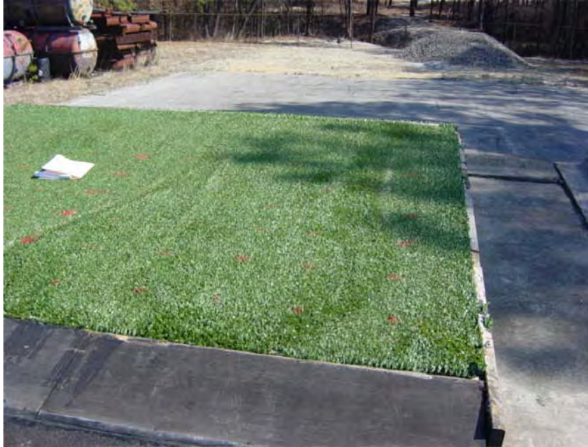
FIGURE C-53. TEST 8—1.5-INCH FIBER TEST PLOT AFTER TESTS
