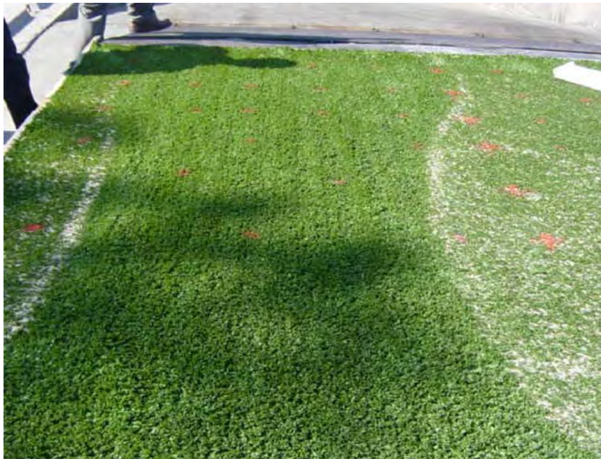
FIGURE C-54. TEST 8—1.5-INCH FIBER TEST PLOT AFTER TESTS, CLOSE-UP
