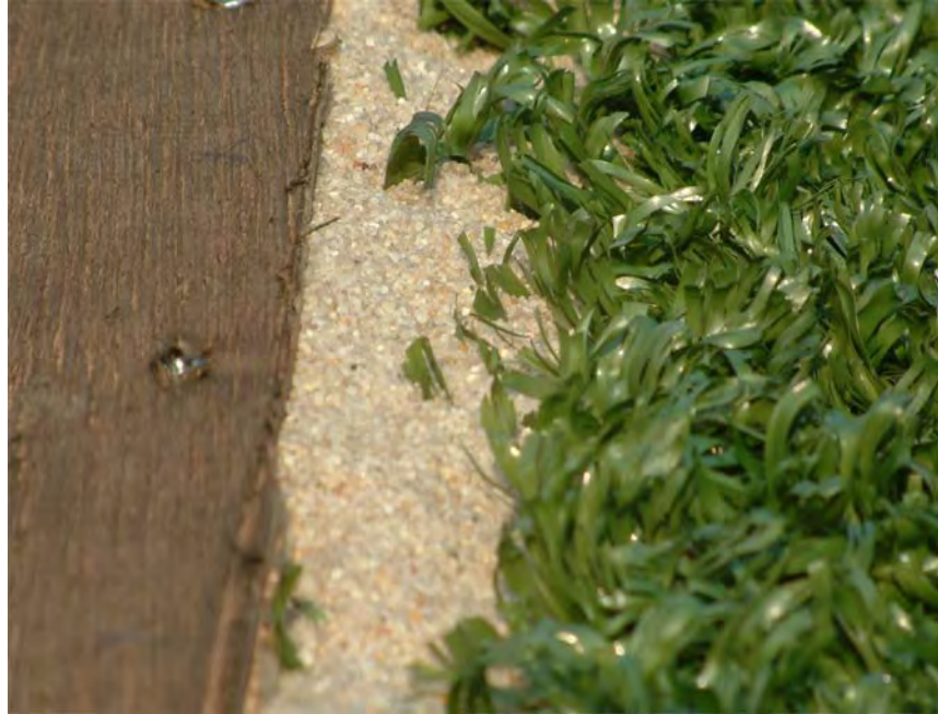
FIGURE C-20. BALLAST SAND INFILL SIDE OF TEST PLOT
