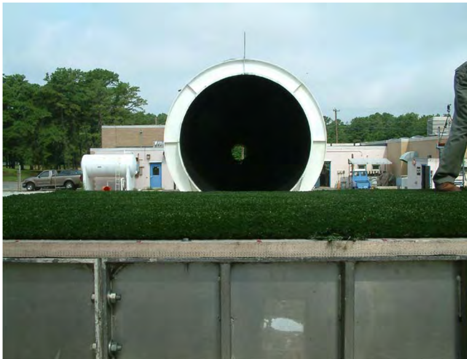
FIGURE C-1. TEST PLOT INSTALLED AT THE FAA WILLIAM J. HUGHES TECHNICAL CENTER WIND TUNNEL
