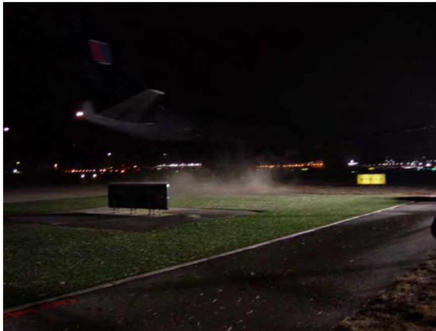
FIGURE 4-16. BOEING 747 TAXIING FROM ARTIFICIAL TURF TO NATURAL GRASS (JET BLAST TEST ACROSS ARTIFICIAL TURF SURFACE) (SFO)
