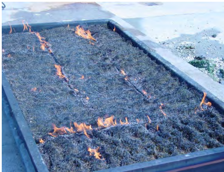
FIGURE D-7. NATURAL GRASS FIRE—ONLY SEAMS INVOLVED
