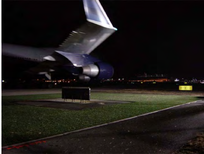
FIGURE 4-15. BOEING 747 TAXIING BY ARTIFICIAL TURF (JET BLAST TEST ACROSS ARTIFICIAL TURF SURFACE) (SFO)
