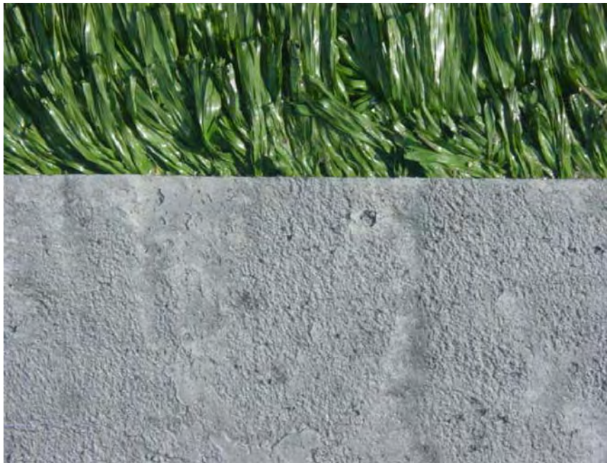
FIGURE C-40. THE 2.0-INCH FIBER WITH QUICK-DRYING CONCRETE HEADER
