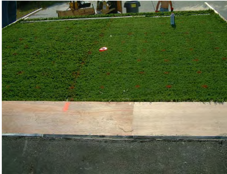
FIGURE C-18. TEST 2b—2.5-INCH FIBER TEST PLOT (SECOND INSTALLATION)
