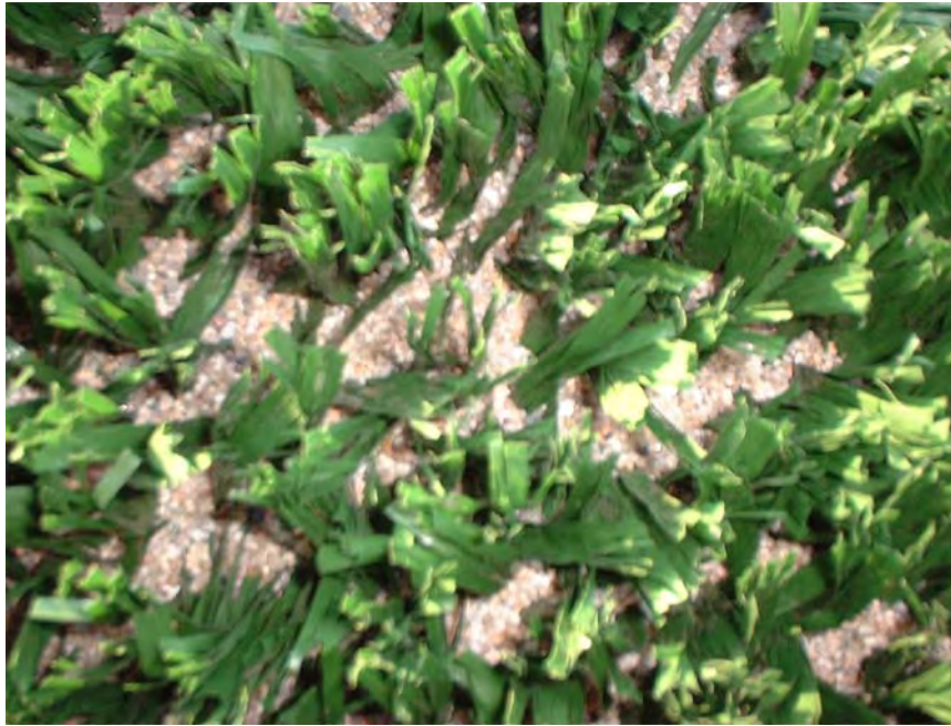
FIGURE 3-6. CLOSE-UP VIEW OF ARTIFICIAL TURF WITH BALLAST SAND, TOP VIEW
