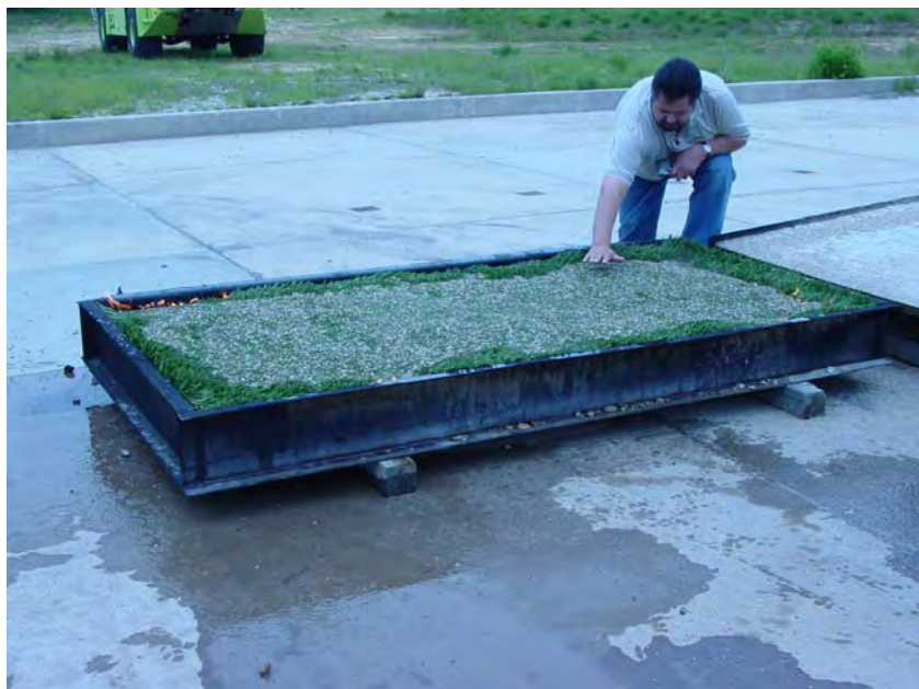
FIGURE D-26. DAMAGE TO MATERIAL AFTER A SHORT BURN (1:30)
