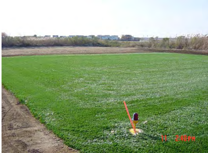
FIGURE 2-18. TEST PLOT LOCATION AFTER ARTIFICIAL TURF INSTALLATION IN RUNWAY SAFETY AREA
