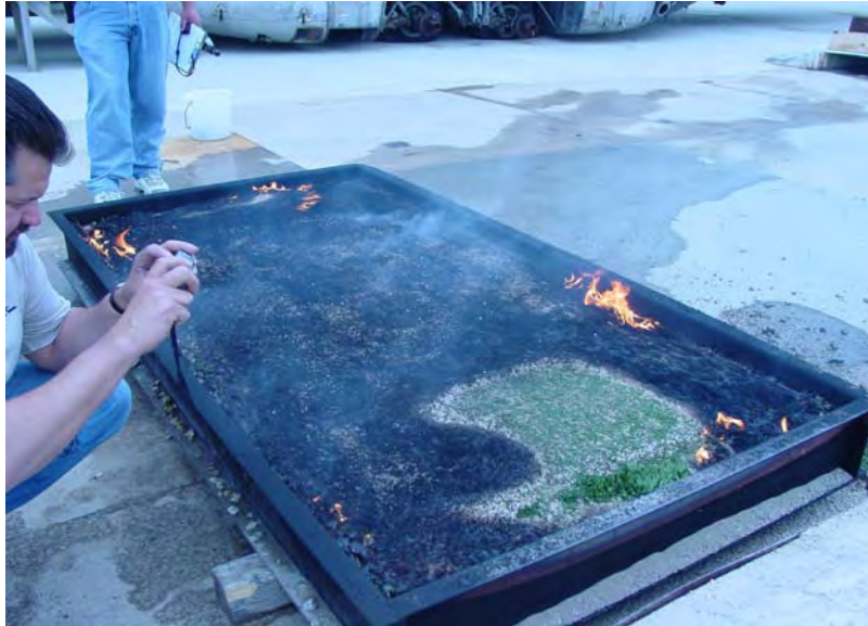
FIGURE D-27. DAMAGE TO MATERIAL AFTER A LONG BURN (28:00)
