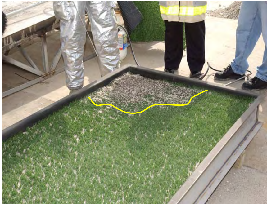
FIGURE D-3. BURNT AREA (OUTLINED IN YELLOW) FROM PROPANE TORCH
