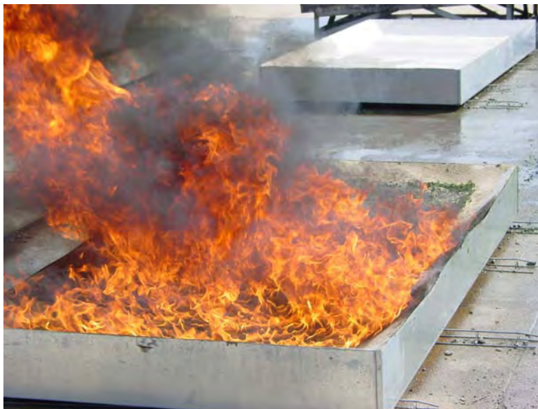
FIGURE D-32. DEMONSTRATION WITH 1-INCH SAND INFILL
