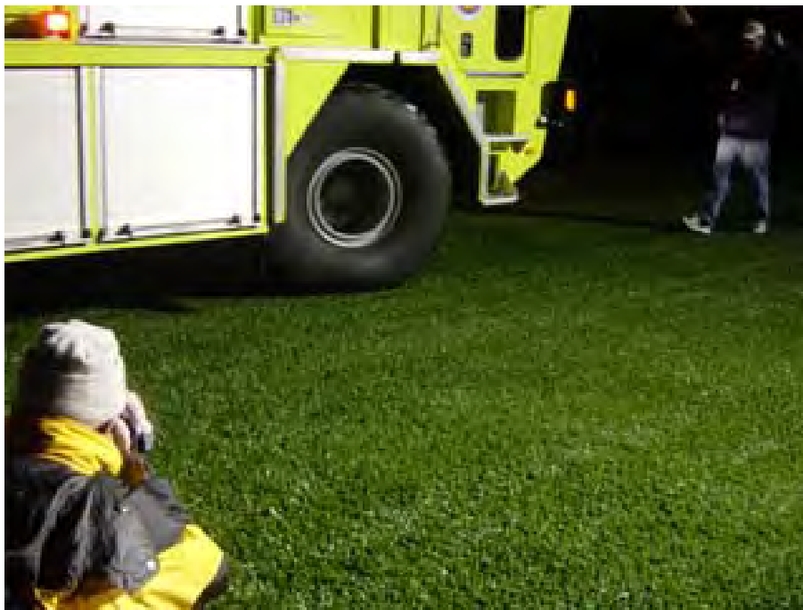
FIGURE 4-1. AN ARFF VEHICLE CONSTANTLY TURNING WHEELS ON ARTIFICIAL TURF SURFACE (BOS)
