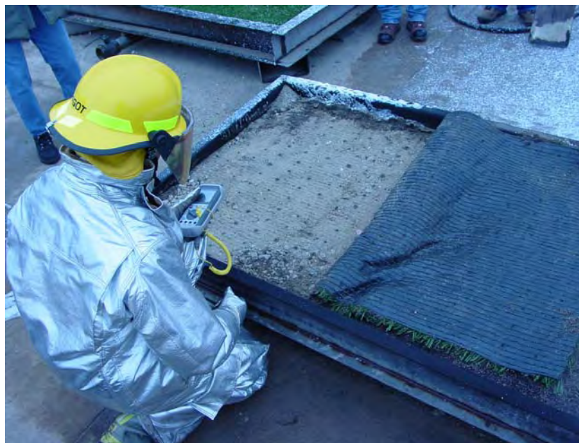
FIGURE D-11. POSTFIRE INSPECTION OF TURF AND BASE MATERIAL
